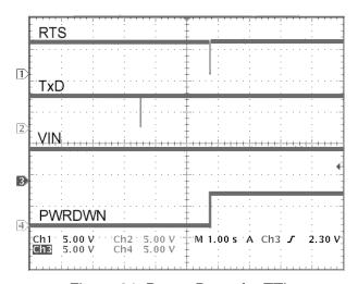
Figure 24. Power Down for TTL
